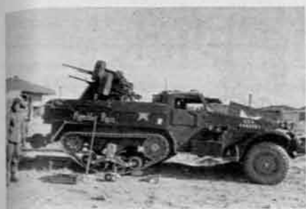
One of the M16's of the author's battery being repaired near Suwon, Korea, after its track had been damaged by a road mine. This is typical of roadside repairs made by the unit.
